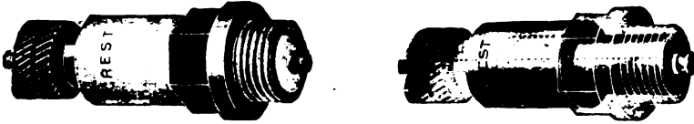
FIG. 330.—The "Crest" Jump-Spark Plug for use in Vehicle Motors. As shown in the half-sectional view, the plug consists of two essential parts; the shell having a thread at one end to screw into an orifice in the combustion chamber, and carrying one terminal of the sparking circuit as shown. Through the inside of the shell is a tapered hole, in which an insulated cone is fitted gas tight. Through this insulation is inserted the other terminal of the circuit, which is a metal knob. This is in electrical contact with the wire screwed to the binding post at the end of the insulated tube. The other terminal is connected to the metal of the cylinder.
